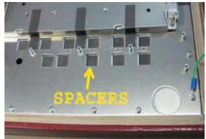
Because of differences in hight of buttons there is a need of an additional spacer with the blue button keyboard
